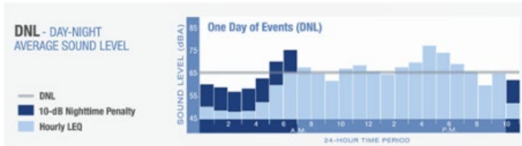
Figure 23: Hourly Sound Levels in dBA Illustrating the 10 dB Penalty Applied During Evening Hours
